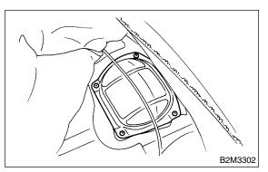
10) Disconnect connector from fuel pump.
