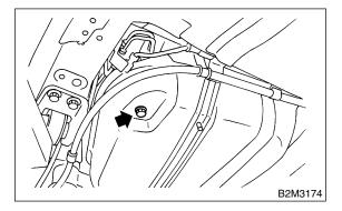
7) Tighten fuel drain plug and install front right side fuel tank cover.
