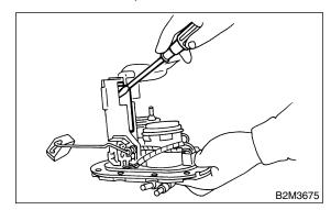
2) Disconnect connector from fuel pump.
