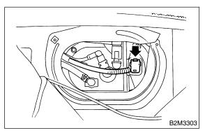
11) Move clips and then disconnect jet pump hose (C).
