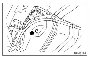
5) Tighten fuel drain plug and install front right side fuel tank cover.
