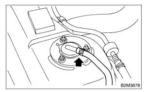
3) Remove bolts which install fuel cut valve.
