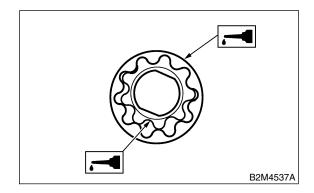
2) Install the inner rotor by fitting it into the groove on the crankshaft, and then assemble the outer rotor.
