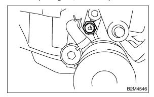
3) Connect terminal of oil pressure switch.
