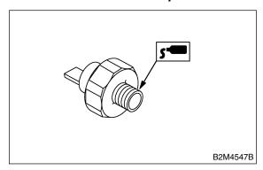
2) Install oil pressure switch.
