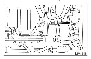
6) Remove oil pressure switch.
