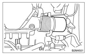
8) Remove connector and remove oil cooler.
