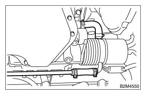
4) Install water pipe to engine.
