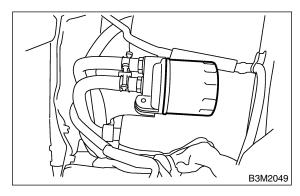
4) Get new ATF filter and apply a thin coat of ATF to the oil seal
