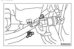
4) Remove oil filter bracket installation nut.
