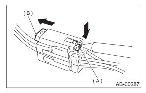
(2) Then separate the connector halves by pulling them apart while pressing lever (A).
