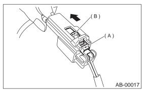
3) With slide lock (B) pulled, remove lock arm (A) to its original position, and then pull in the direction of the arrow and separate the connector.
