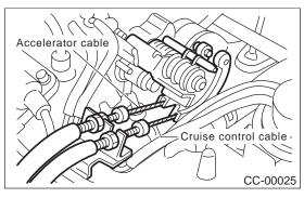
Check the cruise control cable installation. If NG, install the cable securely.
