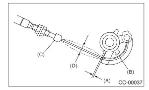
Check that the clearance (A) between throttle cam (B) and lever or cable deflection (D) is within specifications.
