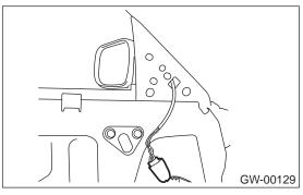
3) Loosen screws to remove mirror assembly.
