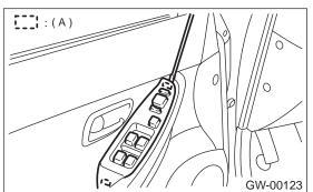
2) Remove four hook (A) to remove remote control mirror switch.
