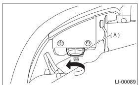
5) Remove spring retainer then detach fog light bulb.
