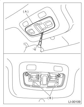
3) Disconnect harness connectors and remove spot light.
