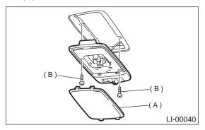
3) Disconnect harness connectors and remove the light.
