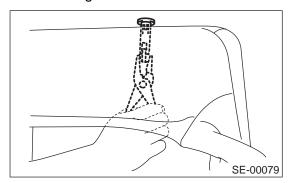
10) Remove hog ring (A) on front face of seat.
