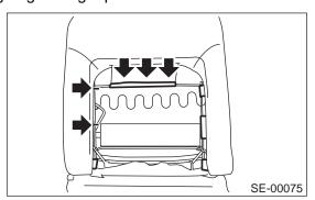
5) Remove clamp of side airbag wire harness. (Side airbag equipped vehicle)
