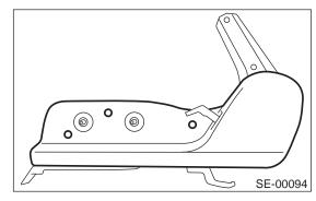
26) Remove seat hinge cover and hinge spring cover.
