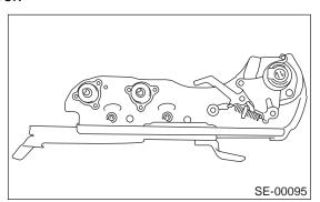
27) Remove 2 bolts, and then remove slide rail.
