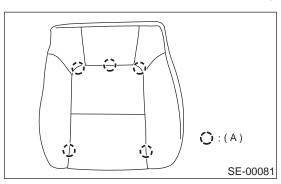
11) Remove hog rings, and then remove seat heater. (Seat heater equipped vehicle)
