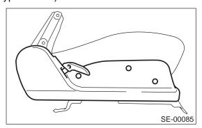
17) Remove the 4 bolts of seat hinge assembly, and then remove seat cushion.
