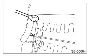
16) Remove reclining cover and hinge cover. (Non-tilt type vehicle)
