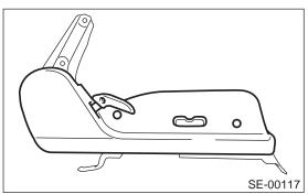
24) Remove the cover on the underside of the seat hinge, remove the two bolts, and remove the seat hinge.
