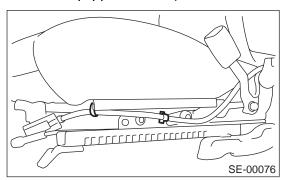
7) Turn cover and cushion, and remove the two bolts from hinge.
