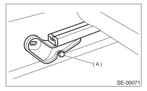
3) Tighten the four bolts of slide rail.
