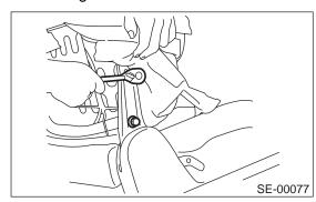
8) Remove hinge screw cover and screws, and remove seat back from hinge.
