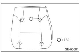
11) Remove wire rings, and then remove seat heater. (Seat heater equipped vehicle)
