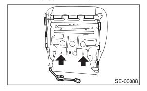
20) Remove hog rings (A). Tilt type vehicle:
