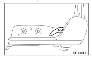
25) Remove hinge cover cap and screws.
