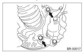
3) Remove the disc rotor.
