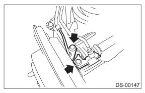
9) Adjust parking brake lever stroke by turning adjuster. <Ref. to PB-5, ADJUSTMENT, Parking Brake Lever.>
