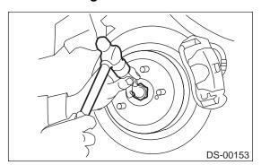
11) Install wheel and tighten wheel nuts to specified torque.
