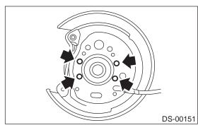
2) Tighten four bolts to back plate.
