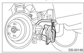
8) Remove disc rotor from hub.
