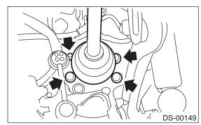
10) Remove hub unit bearing.
