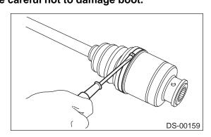
3) Remove circlip from SFJ outer race using screwdriver.
