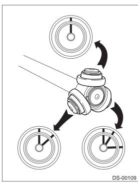
15) Align alignment marks on shaft and outer race, and install outer race.
