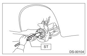
3) Tighten axle nut temporarily.
