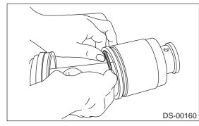
4) Remove SFJ outer race from shaft assembly.5) Wipe off grease.
