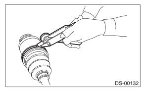
22) Tap on the clip with the punch provided at the end of ST.
