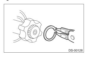
5) Install cage, which was previously fitted, to inner race fixed upon shaft.
