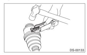
17) Cut off band with an allowance of about 10 mm (0.39 in) left from the clip and bend this allowance over the clip.
