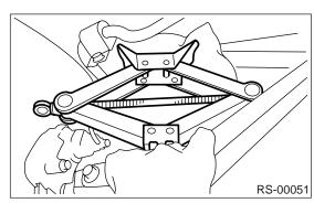
4) Using transmission jack, support rear arm horizontally and tighten shock absorber nuts and bolts to specified torque.
