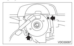
4) Tighten bolts which install roll connector and steering angle sensor onto steering column.
