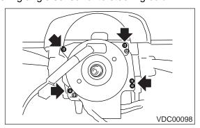
5) Set steering wheel to neutral and install it onto steering shaft.
