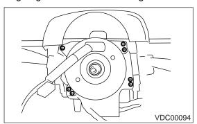
8) Remove roll connector and steering angle sensor
