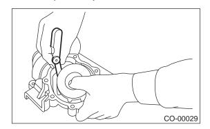
5) After water pump installation, check pulley shaft for engine coolant leaks. If leaks are noted, replace water pump assembly.
