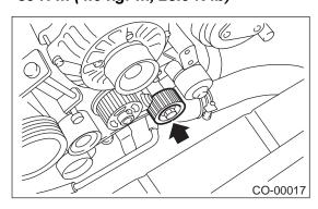
6) Install automatic belt tension adjuster which tension rod is held with pin. <Ref. to ME(H4SO)-47, AUTOMATIC BELT TENSION ADJUSTER AS-SEMBLY AND BELT IDLER, INSTALLATION, Timing Belt Assembly.>
