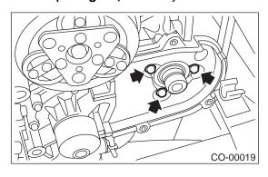
4) Install left-hand camshaft sprockets by using ST. ST 18231AA010 CAMSHAFT SPROCKET WRENCH
