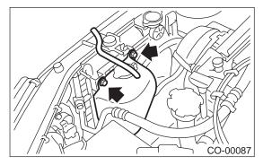
11) Remove radiator main fan and sub fan assemblies. <Ref. to CO(H4SO)-27, REMOVAL, Radiator Main Fan and Fan Motor.> and <Ref. to CO(H4SO)-29, REMOVAL, Radiator Sub Fan and Fan Motor.>
