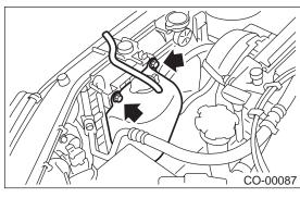
12) Disconnect radiator inlet hose from engine.
