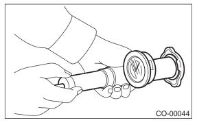
2) Increase pressure until tester gauge pointer stops. Radiator cap is functioning properly if it holds the service limit pressure for five to six seconds.
