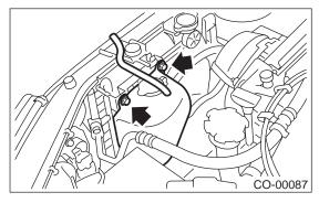
9) Remove radiator main fan motor assembly.
