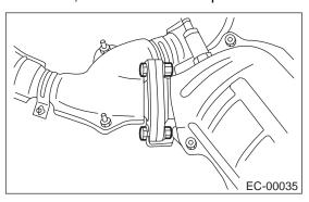
1) Install front and center exhaust pipes. <Ref. to EX(H4SO)-6, INSTALLATION, Front Exhaust Pipe.>
