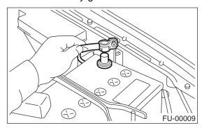
2) Remove bolt which installs purge control solenoid valve onto intake manifold.
