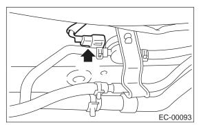
5) Disconnect two evaporation hoses from pressure control solenoid valve.
