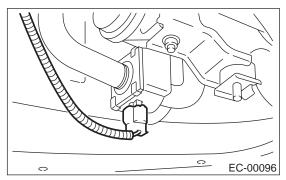
6) Remove bolt which installs drain filter and drain valve brackets on body.
