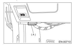
3) Using the OBD-II general scan tool, call up diagnostic trouble code(s) and freeze frame data. OBD-II general scan tool functions consist of:
