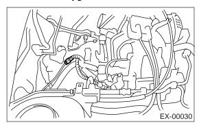
10) Connect front oxygen (A/F) sensor connector.
