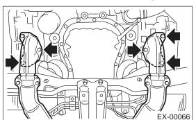
4) Tighten nuts which hold front exhaust pipe onto cylinder heads.
