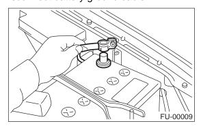
2) Disconnect front oxygen (A/F) sensor connector.
