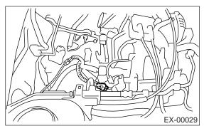
3) Disconnect rear oxygen sensor connector.
