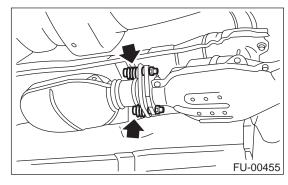
2) Separate rear exhaust pipe from muffler.
