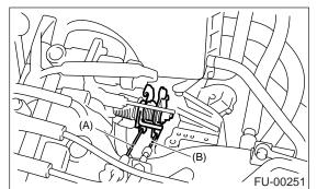
5) Disconnect connectors from idle air control solenoid valve, throttle position sensor and pressure sensor.
