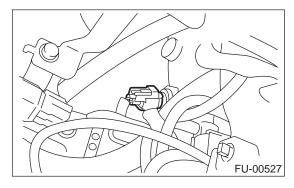
4) Remove engine coolant temperature sensor.
