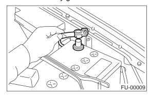
2) Disconnect connector from pressure sensor.
