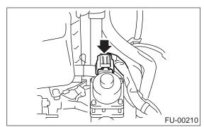
3) Remove EGR valve from intake manifold.
