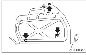
5) Remove nuts (A) which hold ECM to bracket.6) Remove clip (B) from bracket.
