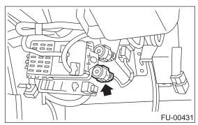
4) Remove fuel pump relay from mounting bracket. **B: INSTALLATION**
