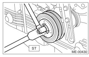
3) Remove crankshaft pulley.
