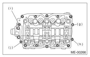
(3) Install valve rocker assembly.
