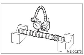
2) Check journal for damage and wear. Replace if faulty.
