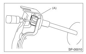
13) Separate accelerator cable and bracket.
