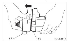
10) Remove clutch (A) from housing (B).
