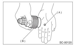
12) Remove idle gear (A) from housing.
