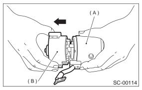
6) Remove brush (A) by lifting up positive (+) side brush spring (B) using long-nose pliers.
