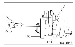
9) Remove housing (A) from magnetic switch (B).
