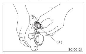
13) Remove retainer and roller (A) from housing.
