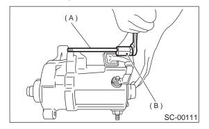
3) Remove yoke (A) from magnetic switch (B).
