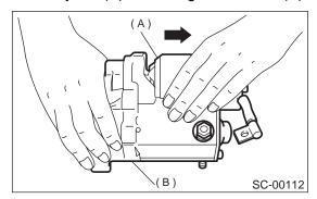
4) Remove screws (A) securing brush holder to end frame (B).
