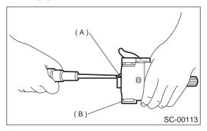
5) Separate yoke (A) from end frame (B).
