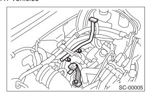
4) Disconnect connector and terminal from starter.
