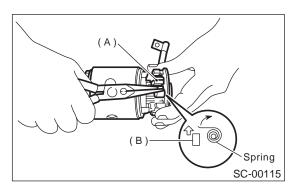
7) Remove armature (A) from yoke (B).
