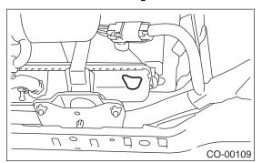
4) Disconnect radiator outlet hose from thermostat cover.
