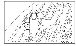
2) Apply a pressure of 157 kPa (1.6 kg/cm<sup>2</sup>, 23 psi) to radiator to check if:
