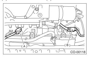
6) Disconnect radiator outlet hose from radiator.
