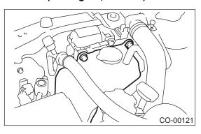
7) Install air intake duct.
