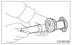
2) Increase pressure until tester gauge pointer stops. Radiator cap is functioning properly if it holds the service limit pressure for five to six seconds.
