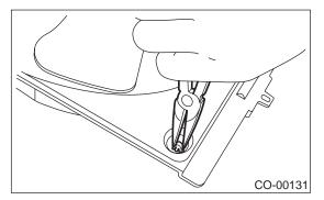
2) Remove nut which holds fan itself onto fan motor and shroud assembly.
