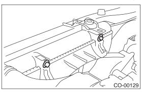
12) Remove radiator main fan motor assembly.
