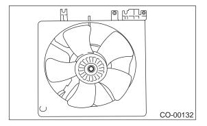
3) Remove screws which install fan motor onto shroud.
