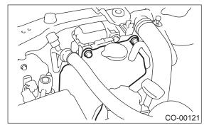
10) Disconnect radiator inlet hoses from radiator.
