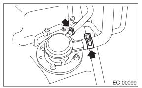
3) Remove nuts which install vent valve on fuel tank.
