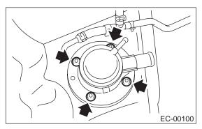
C: INSPECTION Make sure that hoses are not cracked or loose.
