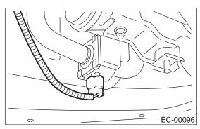
6) Remove bolt which installs air filter and drain valve brackets on body.
