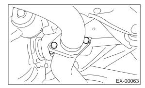
2) Install rear exhaust pipe to front exhaust pipe.
