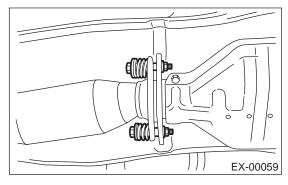
2) Separate rear exhaust pipe from muffler.
